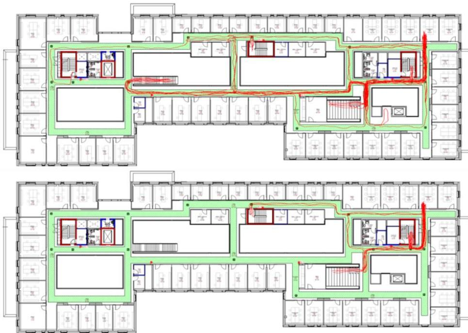
Figure 4 The upper floorplan shows the test person's evacuation route, on the 3<sup>rd</sup> floor before changes were made to the VR. The lower floorplan illustrates the evacuation route test persons took on the 3<sup>rd</sup> floor after changes were made to the VR.
