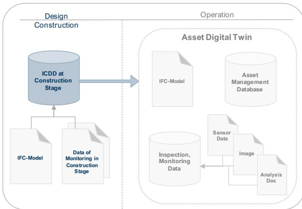
Figure 1: Overview of the information flow of as-built data between the construction and operation phase for asset management
