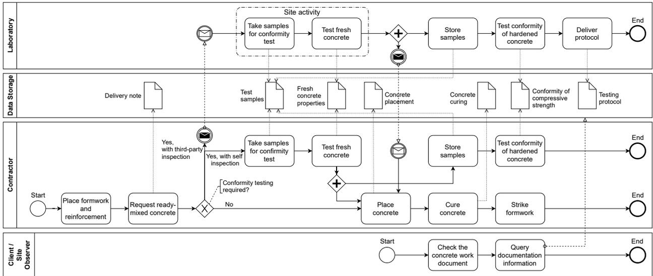
Figure 3: Process map of concreting and documentation with information exchange
