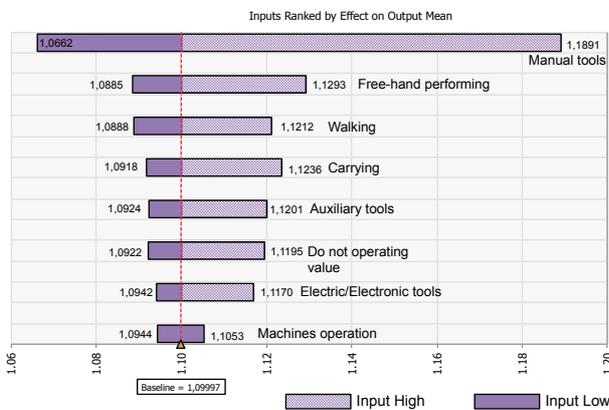
Figure 2: Masonry (residential) process sensitivity analysis
