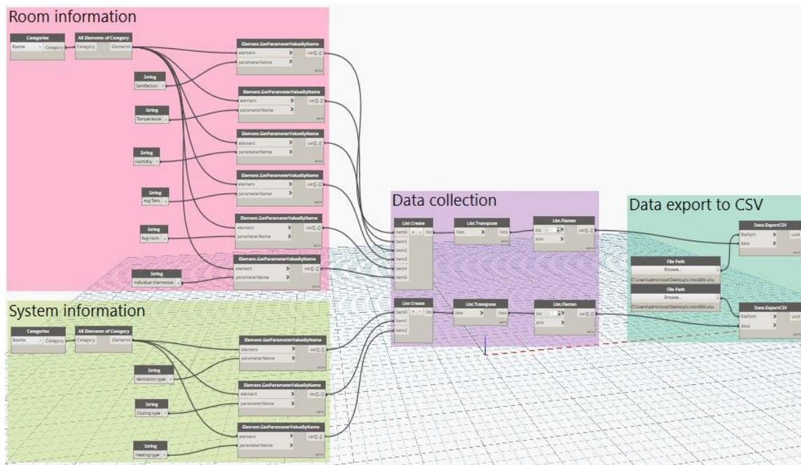
Figure 2: Dynamo script used for data extraction
