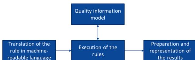
Figure 5: Process of quality compliance checking adapted from (Eastman et al. 2009)
