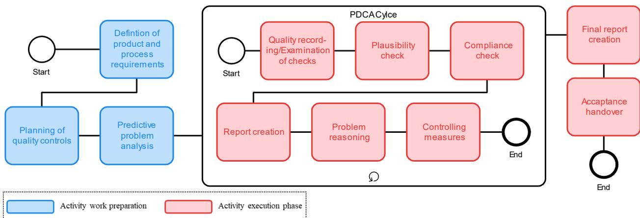
Figure 6: Process diagram of quality management in the construction execution phase
