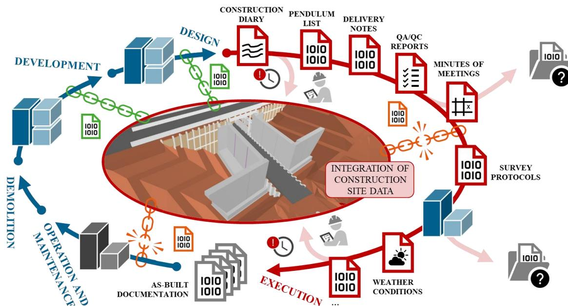
Figure 1: Missing data and information during the information life cycle of a bridge structure
