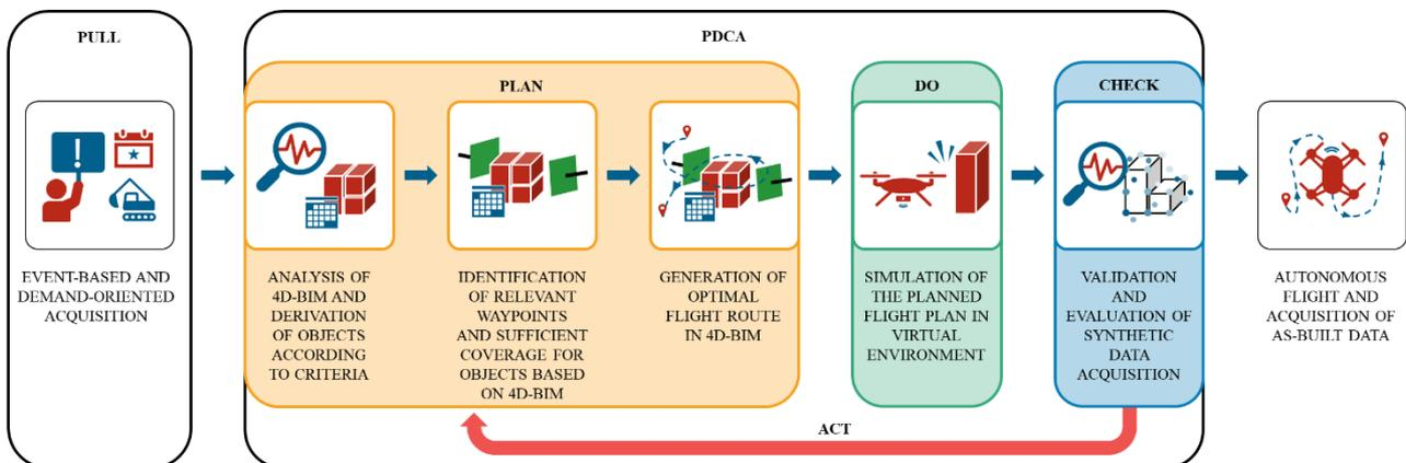
Figure 4: Concept for the lean data acquisition process (LDAP)
