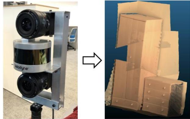
Figure 1: Our prototypic scanner (left); an indoor scene reconstructed using the proposed method (right).
