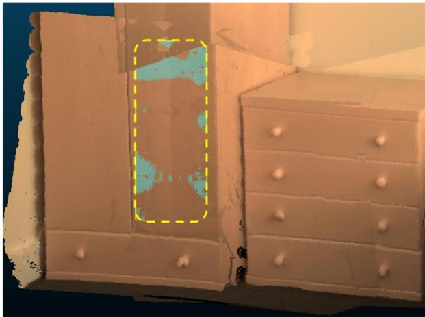
Figure 6: We measure the precision in reconstructing flat surfaces in the place marked with the yellow dashed rectangle. A fit plane there is marked in blue translucent color.
