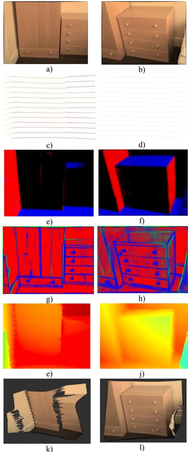
Figure 3: Partial outputs of reconstruction processes outlined in Figure 2. Pairs a) c) and b) d) show time-synchronized undistorted camera images and sparse lidar depth maps; e) and f) portray predicted normal vectors of surfaces; g) and h) represent predicted occlusion boundaries; i) and j) portray regressed dense depth maps; k) and l) show the back-projected depth maps in the form of point clouds
