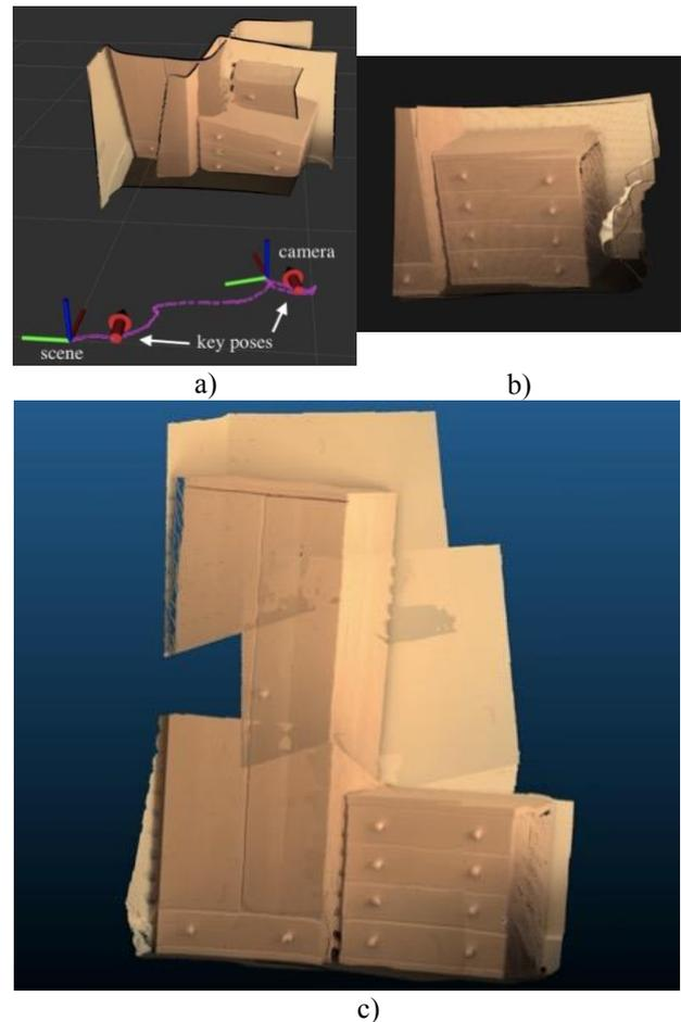
Figure 4: Odometric reconstruction of an indoor scene using our method.
