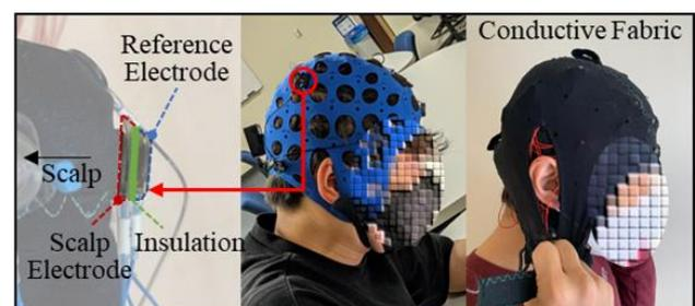
Figure 1: Customized mobile EEG device and details of the paired electrodes
