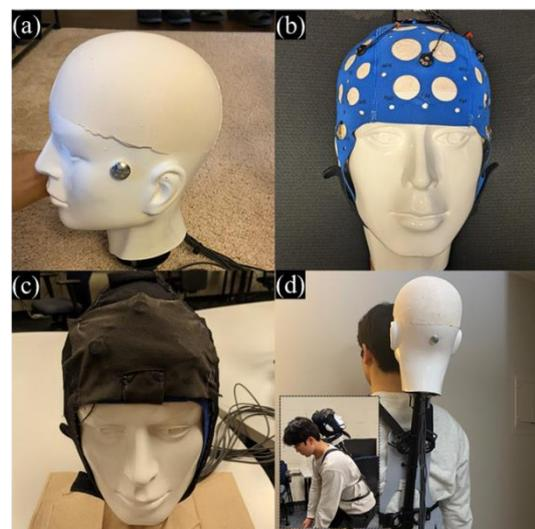
Figure 3. phantom head used in this study; (a) created phantom head; (b) Normal scalp EEG equipped on the phantom head; (c) Paired reference EEG setup; (d) Phantom head worn by a staff
