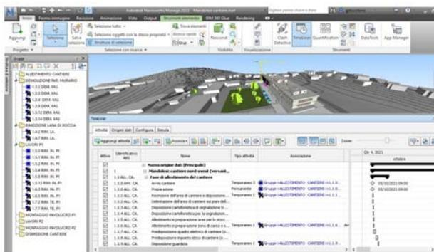
Figure 5: Navisworks Manage - The timeline associated with ABS.
