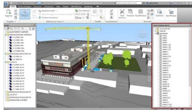
Figure 6: Navisworks Manage - Creating a 4D Simulation.
