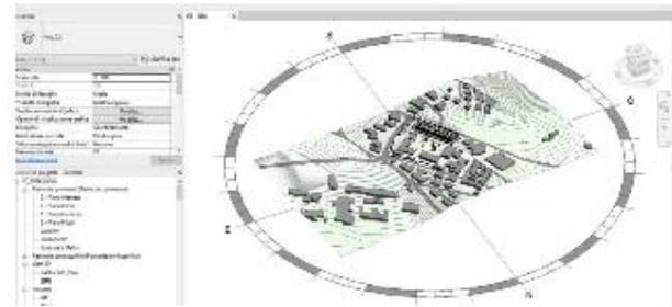
Figure 4: The spatial model extracted from the plug-in and integrated with the building information model and road layout into software Autodesk Revit.
