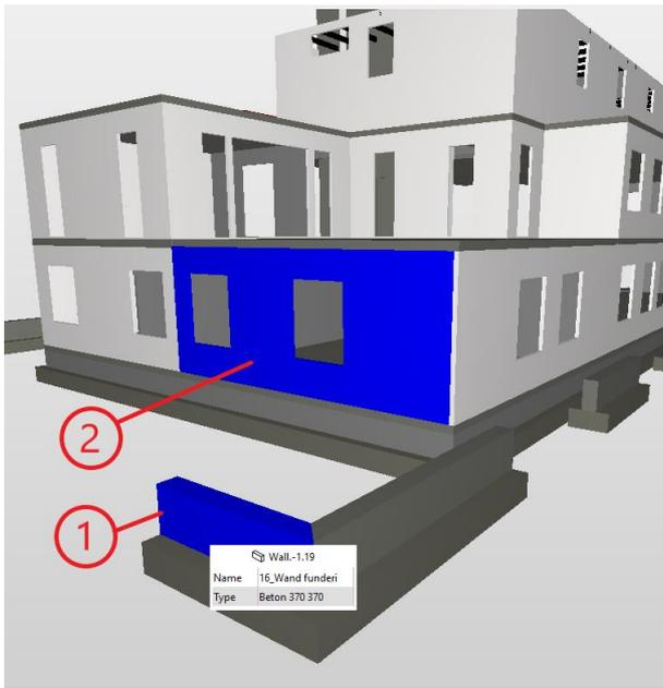
Figure 6. Using IFC-based representations for visual inspection of the building elements
