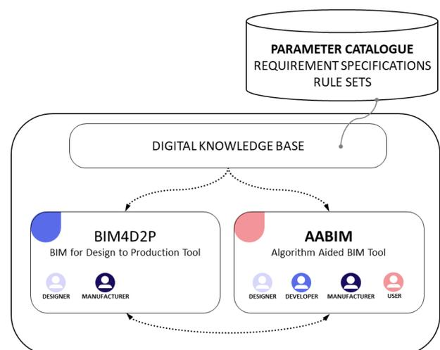
Figure 1: Research Context, Digital Platform Housing 4.0 with its Components: Digital Knowledge Base, BIM4D2P Tool and the Extension AABIM Tool and Parameter Catalogue
