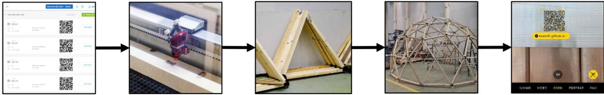
Figure 2. Workflow demonstrating the QR code production, laser engraving, subassembly, main assembly, and accessing the materials passport in situ
