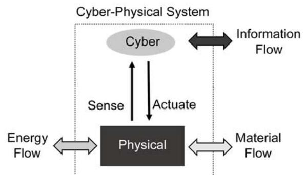
Figure 2: The structure of a Cyber Physical System.
