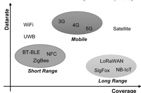
Figure 4: A comparison between several transmission technologies for IoT.
