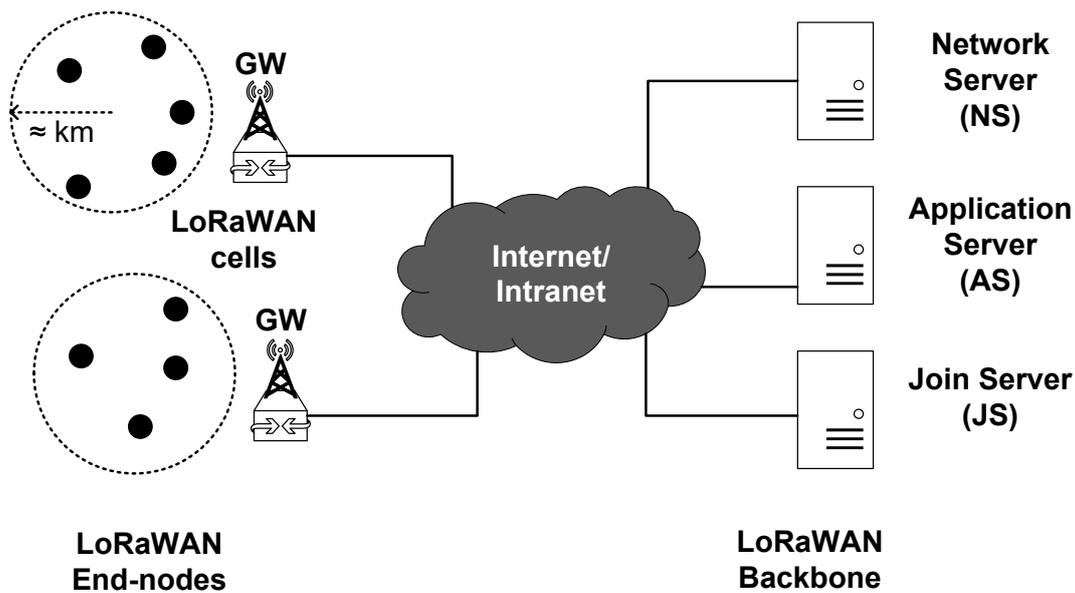
Figure 5: The architecture of a LoRaWAN network.
