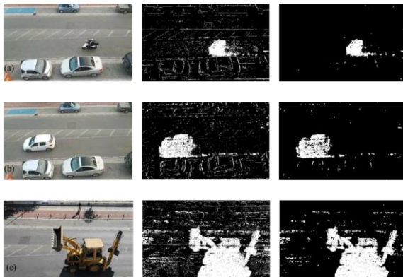
Figure 6: Initial foreground mask and improved foreground mask for: (a) a two-wheeled vehicle; (b) a light vehicle; and (c) a heavy vehicle
