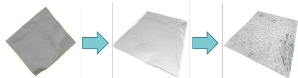
Figure 6: Creating a digital elevation model from point clouds
