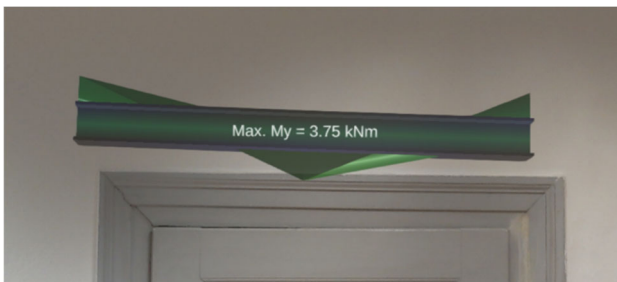
Figure 7: Holographic view of analysis results for bending moments in a beam element with the maximum value
