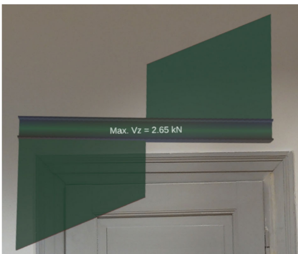
Figure 8: Holographic view of analysis results for shear forces in a beam element with the maximum value
