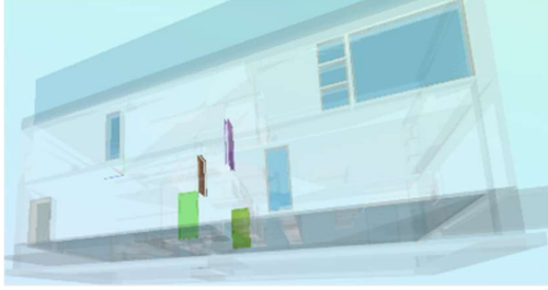
Figure 4: LD-BIM highlighting the four ‘non-compliant’ doors
