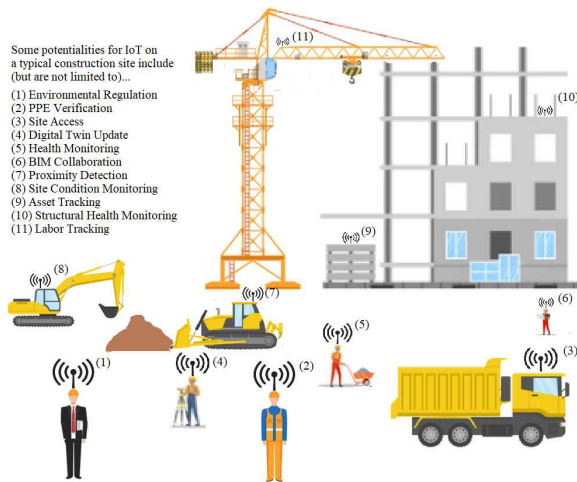
Figure 2: Typical Smart Construction Site Applications (Morman 2021)
