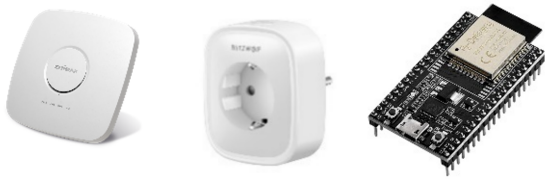
Figure 3: IoT Nodes (Indoor Air Quality sensor, smart plug and custom sensor node)
