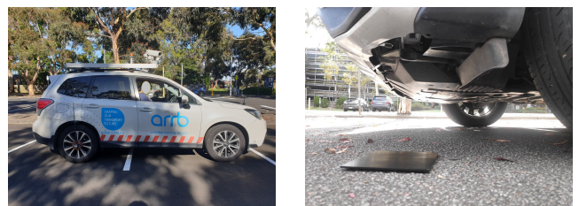
(a) Survey vehicle (b) Profiler (under front bumper) Figure 4: Ground-truth IRI instrument
