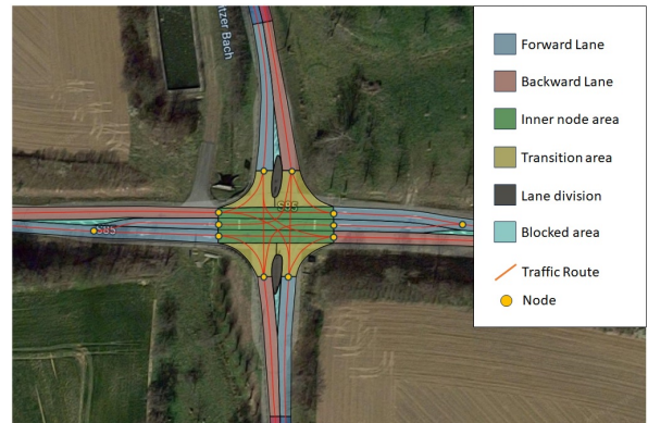
Figure 3: Structure of the microtopology of a traffic junction of two roads (Fig. from Wollschläger (2021) overlaid with the microtopological nodes)
