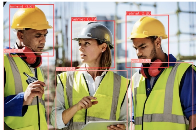
Figure 7: PPE detection of sample in-test photo
