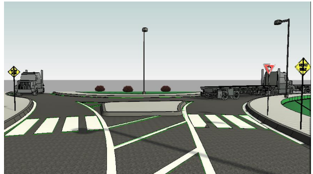
Figure 11: Horizontal marking and vertical signs at roundabout 2
