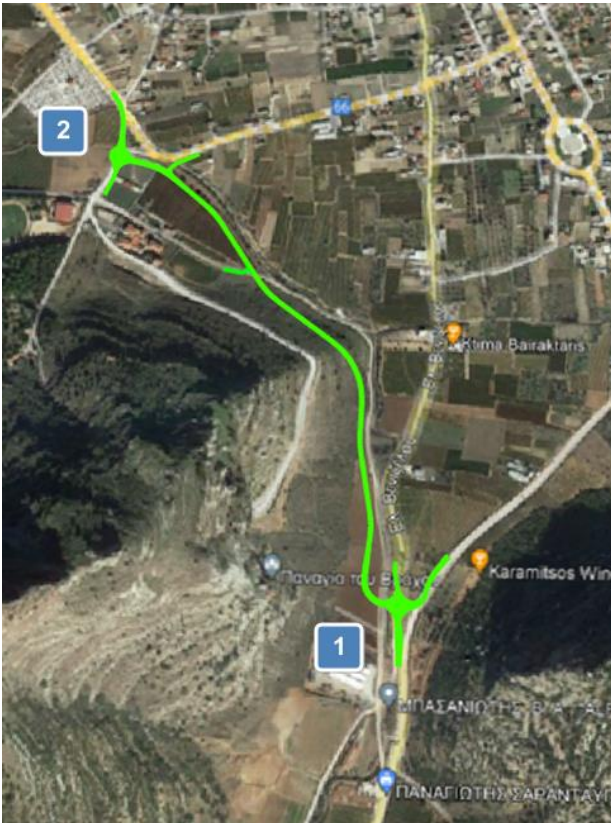
Figure 4: Ring road alignment design
