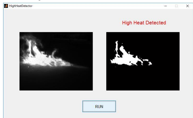
Figure 9: Detection of high heat using thermal imaging
