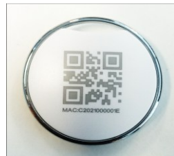
BLE-Beacon placed inside equipment
