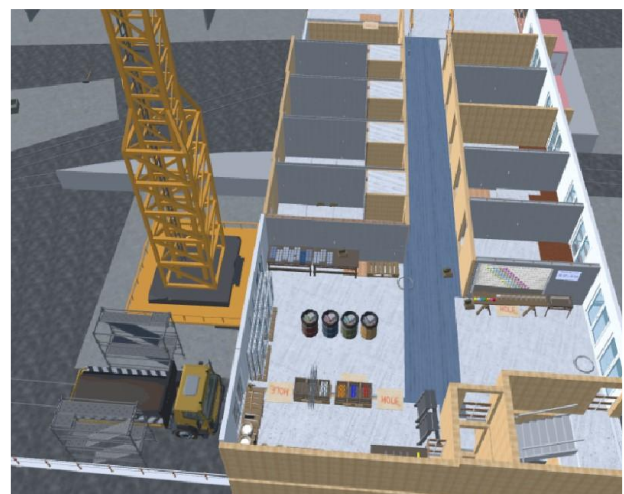
Figure 1. Scene overview of the virtual construction site in Unity with zones highlighted.
