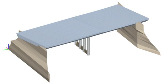
Figure 11: the automated generated parametric BrIM geometry (LOD 300).
