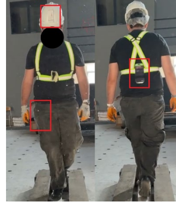
Figure 1: Participant instrumented with a UWB tag (hardhat) and smartphones (pocket and lumbar) for data collection.
