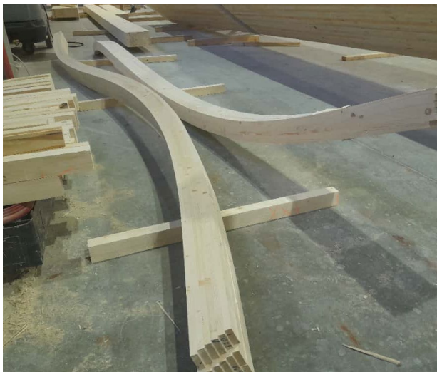
Figure 12 Free-form glulam blank prototypes produced using the digital workflow.
