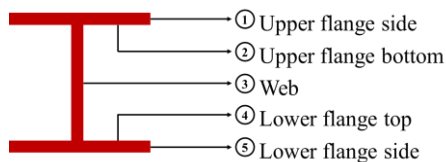
Figure 3: Steel structure beam surfaces
